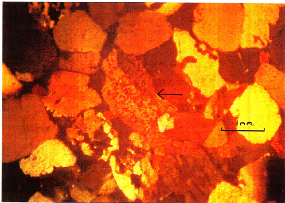
Figure 5-13d Authigenic vermicular kaolinite under cross-nicols
